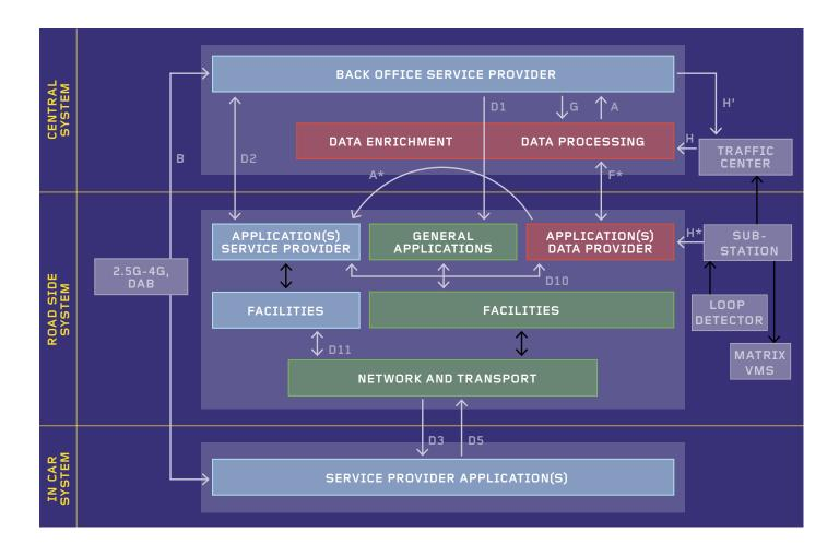
The architecture of the cooperative system from Shockwave Traffic Jams A58, with a schematic diagram of the subsystems (components) and interfaces. The colours indicate which provider is at work: the data provider (red), the service provider (blue), or the communications provider (green). Each role can be played by different parties, which can collaborate and compete.
